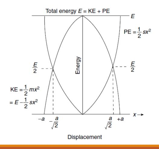
•The solution  $x = a \sin(\omega t + \phi)$ reveals that the total energy of the oscillator must remain constant because the maximum displacement is regained after every half cycle.
