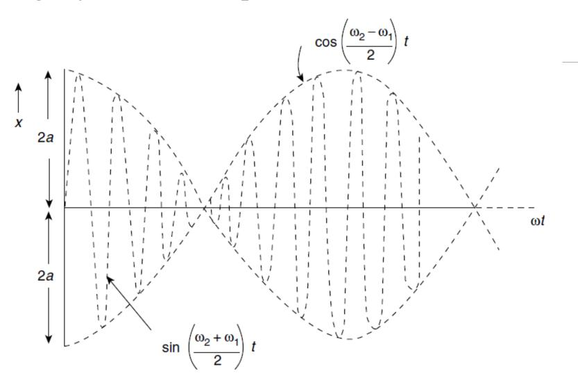
The displacement graph shows the amplitude modulation of the high frequency components
