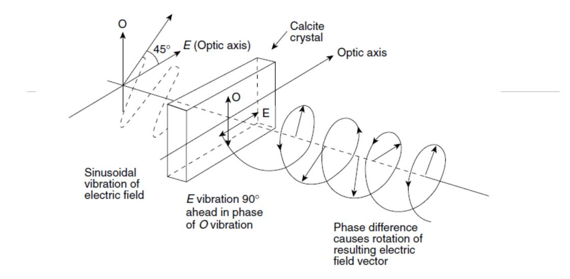
The polarization transformation due to a linear light passing through a birefringence crystal can be determined from the superposition of two perpendicular harmonic vibrations. The final output polarization is a circularly polarized.
