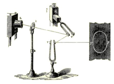
Lissajous' method of calibrating one tuning fork against another. When the two forks gave the same frequency, a beam reflected off both forks and projected on a screen, would form a steady ellipse. An experimental setup made by Jules Antoine Lissajous to study the superposition of two perpendicular vibrations with **different angular frequencies**.
